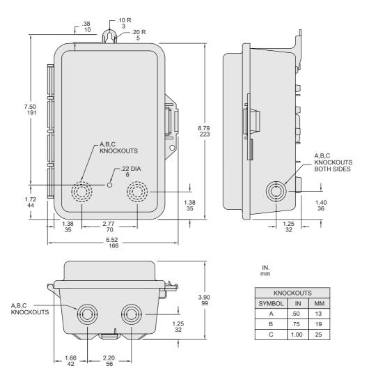
ALL DIMENSIONS ARE APPROXIMATE. REFER TO TECHNICAL DRAWINGS AND DOCUMENTATION WHEN MOUNTING, ALLOW 1.50IN / 38MM CLEARANCE ON HINGE SIDE FOR DOOR TO OPEN.
